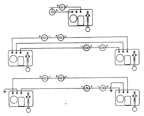
Diagrams for connecting the Johnson Model 450 Practice Set are shown above. Two 1½ volt dry cell batteries for single set operation or four 1½ volt dry cell batteries for operating two sets will be needed to provide electric power.
