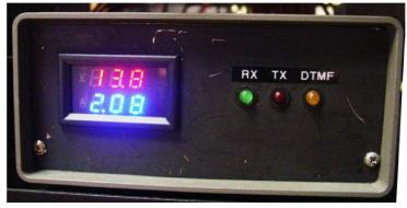
Controller. A Hamtronix Elektra 2000 DTMF controller is used to interface the VHF receiver and transmitter and the UHF link transceiver. Controller functions are described in the manual. The controller is mounted inside a metal enclosure and the LED indicators are remoted to the front panel. Controller level settings are accessible through a slot in the top of the
