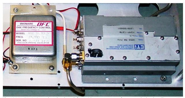
The 10 MHz TCXO pictured on the above left provides an accurate reference to the local oscillator, a CTI XDMP phase locked oscillator module. The +13 dBm output of the XDMP pictured on the right of is
