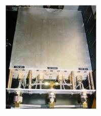
**Duplexer.** A Paladin D1270-4 duplexer connects the single antenna to both receive LNA and transmit PA. The low insertion loss of this duplexer allows the PA to provide almost 30 watts into the feedline.
