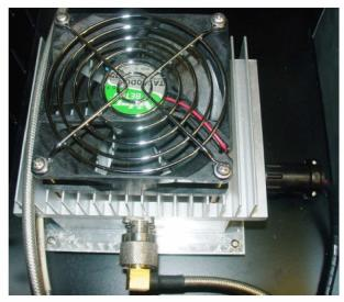
the fan runs only when the repeater is active, a fan timer delay circuit is built into the PA enclosure.
